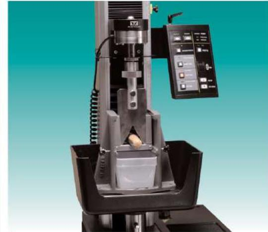
Warner-Bratzler shear fixture with support frame and dip tray
